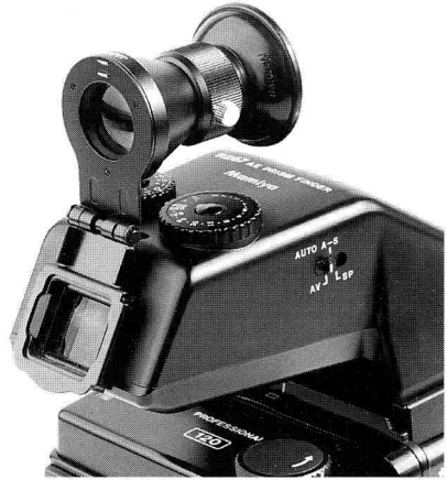
Variable Diopter Magnifier in the "flipped up" position for full screen viewing. Flips down for magnified viewing and adjustable diopter correction
